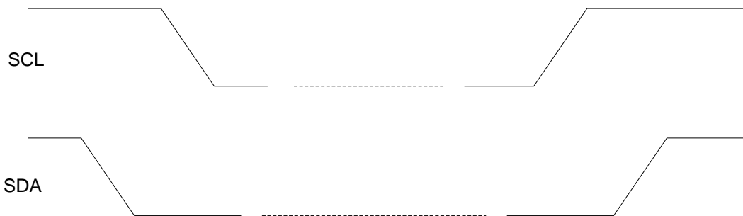
Figure 9: I 2 C START and STOP Condition Timing
