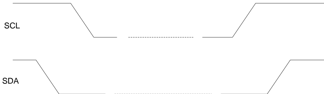
Figure 9: I 2 C START and STOP Condition Timing
