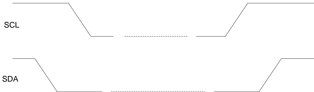
Figure 9: I 2 C START and STOP Condition Timing
