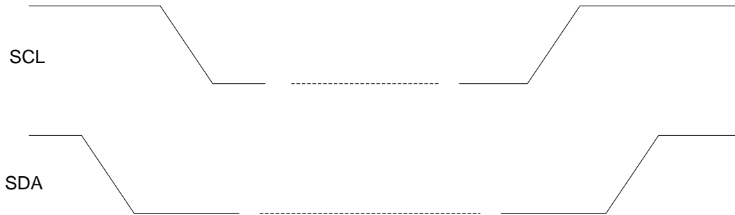
Figure 9: I 2 C START and STOP Condition Timing
