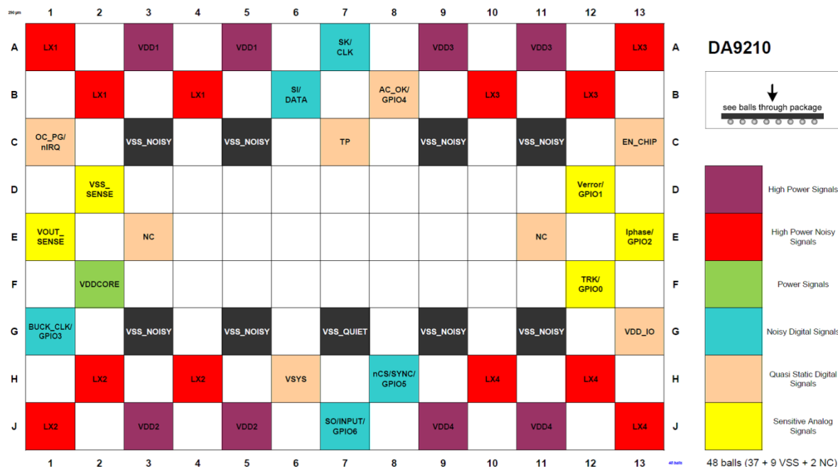
Figure 2: Connection Diagram (48 WLCSP)
