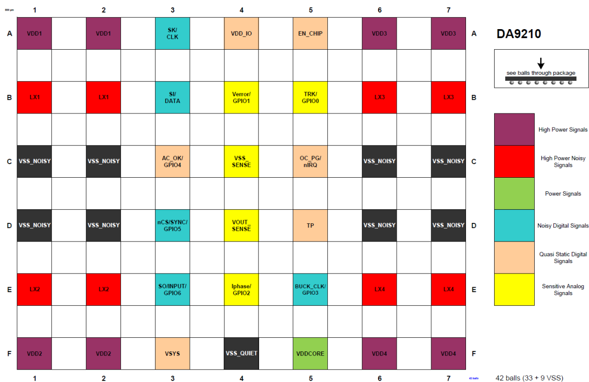
Figure 3: Connection Diagram (42 VFBGA)
