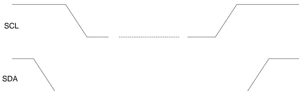
Figure 25: Timing of 2-WIRE START and STOP Condition
