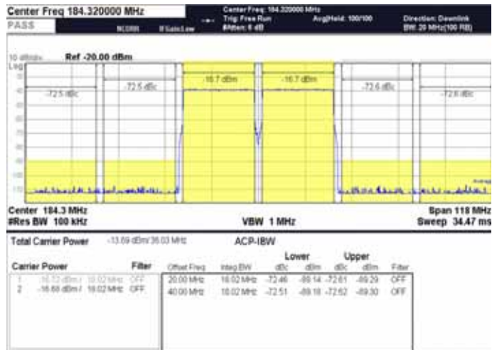
Fig 20. ACLR of 2 carriers LTE (BW=2 x 20 MHz) centered at 184.32 MHz
