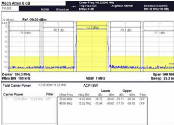
Fig 19. ACLR of 1 carrier LTE (BW=20 MHz) centered at 184.32 MHz
