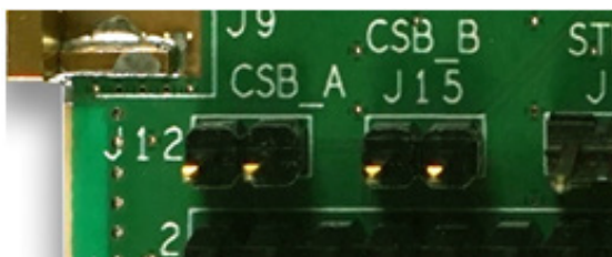
Figure 80. Jumpers for Serial Programming Connections
