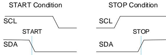
Figure 14. START and STOP Condition Waveform
