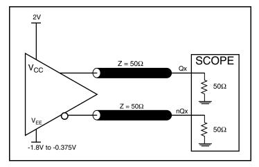
**LVPECL Output Load Test Circuit**
