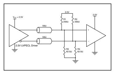
Figure 5A. 2.5V LVPECL Driver Termination Example
