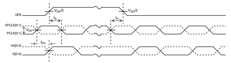
Figure 1. nEN Timing Diagram
