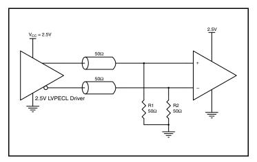
Figure 5C. 2.5V LVPECL Driver Termination Example
