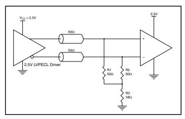
Figure 5B. 2.5V LVPECL Driver Termination Example
