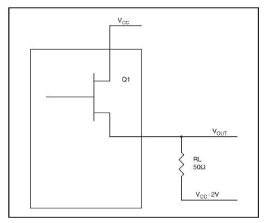
Figure 7. LVPECL Driver Circuit and Termination
