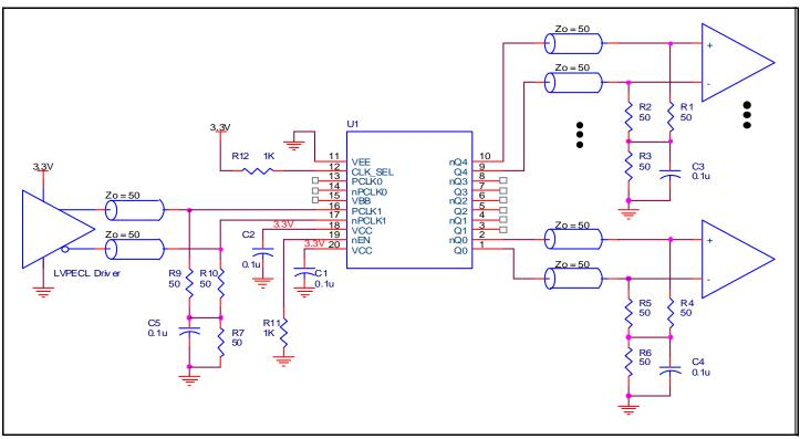
Figure 6. ICS853S014I Example LVPECL Clock Output Buffer Schematic
