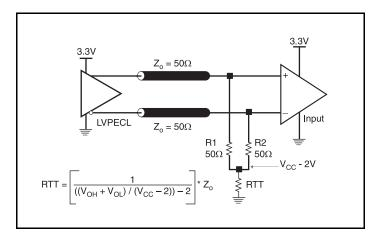
Figure 4A. 3.3V LVPECL Output Termination
