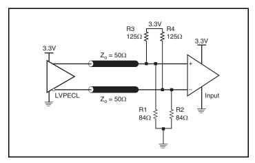
Figure 4B. 3.3V LVPECL Output Termination
