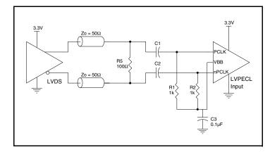
Figure 3F. PCLK/nPCLK Input Driven by a 3.3V LVDS Driver
