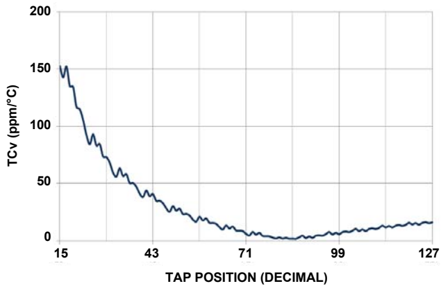
FIGURE 13. 10kΩ TCv vs TAP POSITION, V_{CC} = 3.3V
