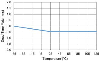
Figure 18. Dead Time Delay vs Temperature; RDU = RDL =  $10k\Omega$
