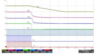
Figure 42. VDD Power-Up Sequence with EN = VDD
