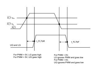
Figure 11. FTLb Propagation Delay (External Driven)
