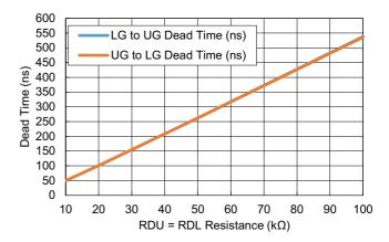
Figure 15. Programmable Dead Time Range  $10k\Omega$  to  $100k\Omega$
