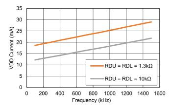
Figure 47. VDD Dynamic Operating Current vs f<sub>SW</sub>; PVCC = BOOT = 4.5V; PHS = GND; No load on UG and LG
