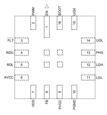
Figure 3. Pin Assignments - Top View
