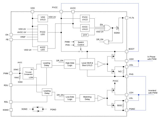
Figure 51. Connection for Dual Low-Side Driver
