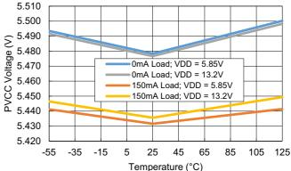
Figure 22. PVCC FB Voltage vs Temperature
