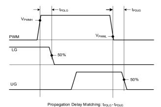
Figure 4. PWM Propagation Delay
