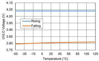
Figure 28. AVCC UVLO vs Temperature
