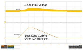
Figure 50. Schottky BOOT Diode Added
