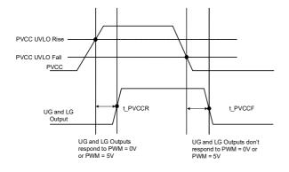
Figure 8. PVCC UVLO to UG & LG Propagation Delay
