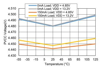
Figure 25. PVCC vs Temperature; PVCC = 4.5V
