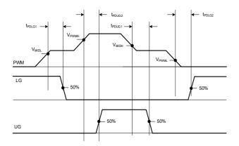
Figure 6. PWM Mid Level Propagation Delay
