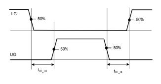
Dead Time Set by Resistor Value on the RDU/RDL Pin Programmable Dead Time Matching:  $t_{DT\_LU}$  -  $t_{DT\_LU}$
