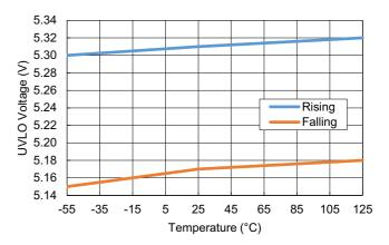
Figure 27. PVCC UVLO vs Temperature
