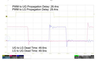
Figure 13. Prop Delay & Dead Time Delay with RDU = RDL =  $10k\Omega$
