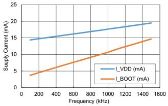
Figure 48. VDD and BOOT Dynamic Operating Current vs f<sub>SW</sub>; VDD = PHS = 12V; PVCC = BOOT-PHS = 4.5V; No load on UG and LG; RDU = RDL= 0V
