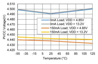
Figure 24. PVCC vs Temperature; PVCC = FB
