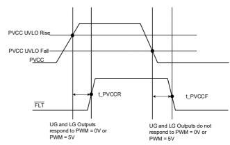
Figure 7. PVCC UVLO to FLT Propagation Delay
