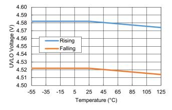
Figure 26. VDD UVLO vs Temperature
