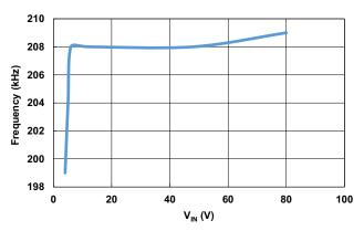
Figure 13. Switching Frequency vs  $V_{IN}$ ,  $R_T = 169k$
