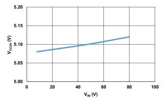
Figure 11.  $V_{CC5V}$  Line Regulation at 20mA Load
