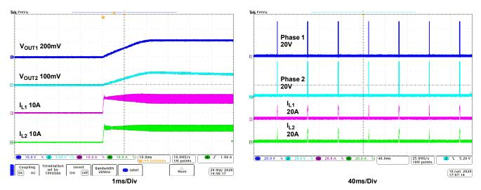
Figure 34. Dual Output Waveforms, Start-Up Waveform,  $V_{IN}$  = 48V,  $V_{OUT1}$  = 12V,  $V_{OUT2}$  = 5V,  $I_{OUT1}$  = 0A,  $I_{OUT2}$  = 0A, CCM
