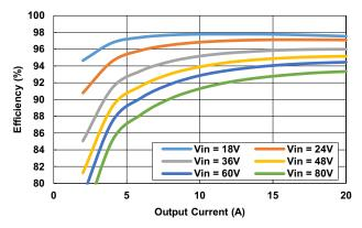
Figure 2. Efficiency (V<sub>OUT</sub> = 12V, CC Mode)
