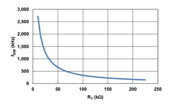
Figure 40. R<sub>T</sub> vs Switching Frequency f<sub>SW</sub>
