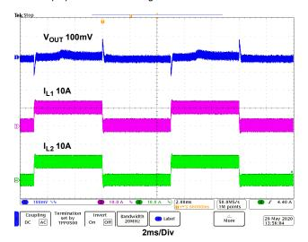
Figure 24. Dual-Phase Waveforms,  $V_{IN}$  = 48V,  $I_{OUT}$  = 0-20A Dynamic, CCM Mode
