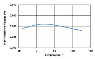
Figure 14. 0.8V Reference Voltage vs Temperature
