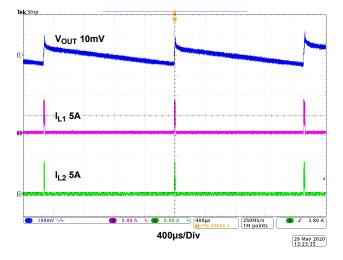
Figure 28. Dual-Phase Burst Mode  $V_{IN}$  = 48V,  $I_{OUT}$  = 0A
