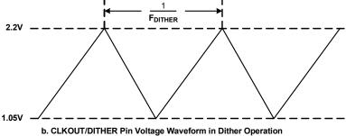
Figure 42. Frequency Dithering Operation
