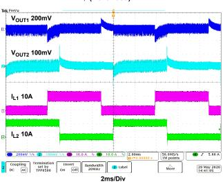
Figure 31. Dual Output Waveform,  $V_{IN}$  = 48V,  $V_{OUT1}$  = 12V,  $V_{OUT2}$  = 5V,  $I_{OUT1}$  = 0-10A,  $I_{OUT2}$  = 0-10A, Dynamic, CCM
