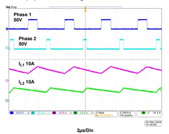
Figure 30. Dual Output Waveform,  $V_{IN}$  = 48V,  $V_{OUT1}$  = 12V,  $V_{OUT2}$  = 5V,  $I_{OUT1}$  = 10A,  $I_{OUT2}$  = 10A CCM
