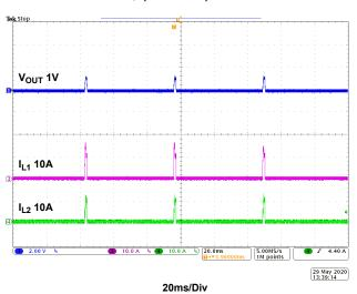
Figure 25. Dual-Phase Waveforms, Burst Mode Waveforms,  $V_{\text{IN}}$  = 48V,  $I_{\text{OUT}}$  = 0.1A
