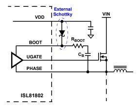
Figure 44. Upper Gate Driver Circuit
