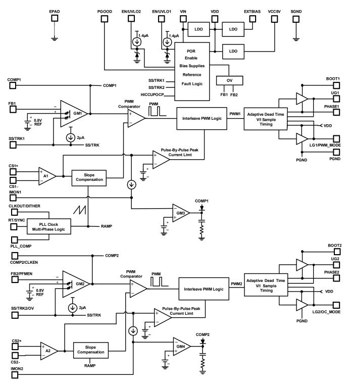
Figure 5. Block Diagram
