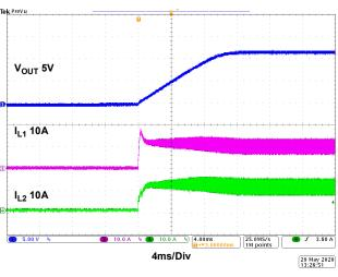
Figure 27. Dual-Phase Waveforms, Start-Up Waveform,  $V_{IN}$  = 48V  $I_{O}$  = 20A, CCM
