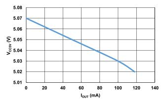
Figure 10.  $V_{CC5V}$  Load Regulation at  $12V_{IN}$
