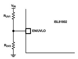
Figure 37. V<sub>IN</sub> Undervoltage Protection
