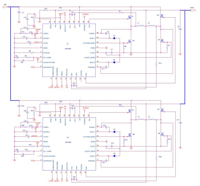
Figure 43. ISL81802 Multi-Phase Current Sharing Circuit
