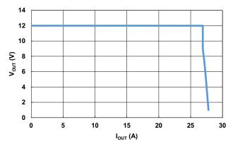
Figure 36. Constant Voltage (CV) and Constant Current (CC) Operation
