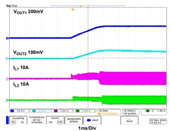
Figure 33. Dual Output Waveforms, Start-Up Waveform,  $V_{IN}$  = 48V,  $V_{OUT1}$  = 12V,  $V_{OUT2}$  = 5V,  $I_{OUT1}$  = 0A,  $I_{OUT2}$  = 0A,  $I_{OUT2}$  = 0A,
