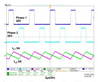
Figure 22. Dual-Phase Waveforms,  $V_{IN}$  = 48V,  $I_{OUT}$  = 0A, CCM Mode
