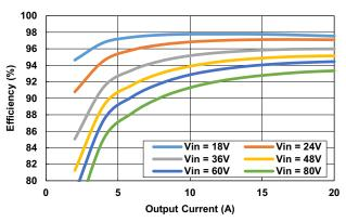
Figure 19. CCM Mode Efficiency
