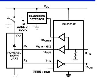
FIGURE 3. DISABLED RECEIVERS PREVENT POWER DRAIN
