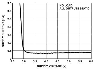
FIGURE 11. SUPPLY CURRENT vs SUPPLY VOLTAGE
