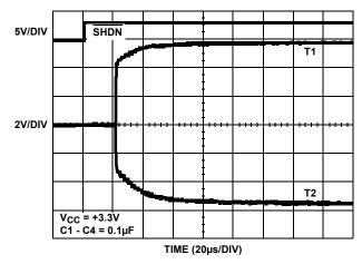
FIGURE 4. TRANSMITTER OUTPUTS WHEN EXITING POWERDOWN
