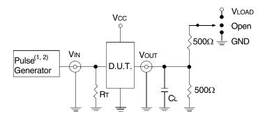
Test Circuits for All Outputs
