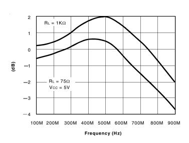
Insertion Loss vs. Frequency
