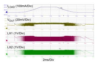
Figure 22. Load Transient:  $V_{IN} = 3.6V$ ,  $V_{OUT} = 3.3V$ , Load Current = 3mA - 400mA Pulsing, US Frequency
