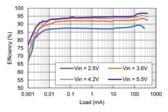
Figure 8. Efficiency vs Load Current:  $V_{OUT} = 5.0V$ ,  $T_A = +25$ °C
