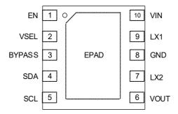
Figure 4. 10 Ld DFN (RAA236100) - Top View
