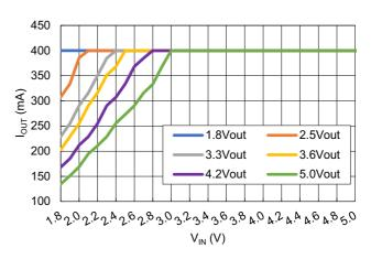
Figure 9. Maximum Load Current vs. Input Voltage
