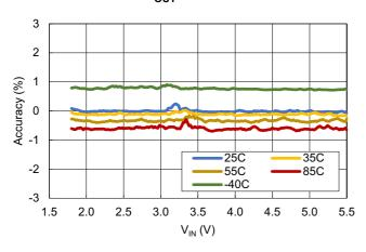
Figure 12. Output Voltage Accuracy vs  $V_{IN}$  vs Temperature,  $V_{OUT} = 3.3V$ , no load
