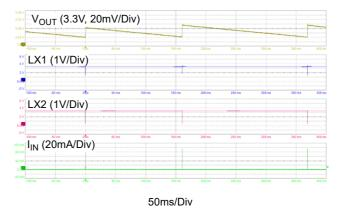
Figure 18. Steady State, PFM mode, Load =  $3.3M\Omega$
