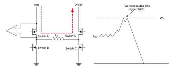
**Figure 30. Overcurrent Protection**
