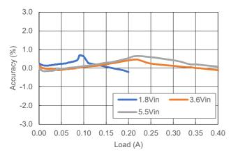
Figure 10. Output Voltage Accuracy vs. Load Current,  $V_{OUT} = 3.3V$
