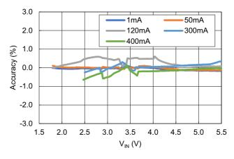
Figure 11. Output Voltage Accuracy vs. Input Voltage, V<sub>OUT</sub> = 3.3V
