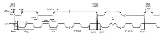
Figure 36. I<sup>2</sup>C Timing
