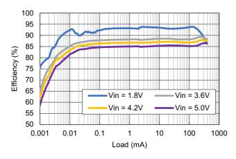
Figure 6. Efficiency vs Load Current:  $V_{OUT} = 1.8V$ ,  $T_A = +25$ °C
