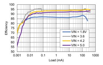
Figure 7. Efficiency vs Load Current:  $V_{OUT}$  = 3.3V,  $T_A$  = +25°C
