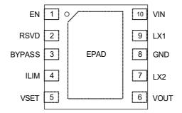
Figure 5. 10 Ld DFN (RAA236105) - Top View
