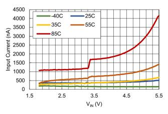
Figure 13. Input Switching Current vs  $V_{IN}$  vs Temperature,  $V_{OUT}$  = 3.3V, no load
