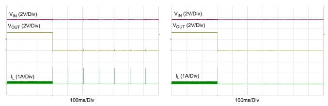
Figure 26. Output Short-Circuit Behavior; Hiccup Mode
