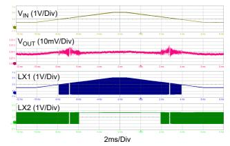
Figure 24. Buck-Boost Transition: V<sub>OUT</sub> = 3.3V; Load = 1mA, PFM mode
