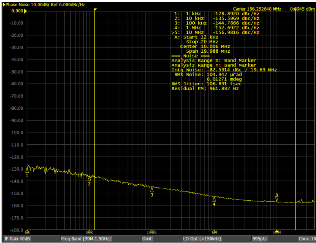
Figure 7. Phase Noise of 156.25MHz Output in Clock Generator Mode
