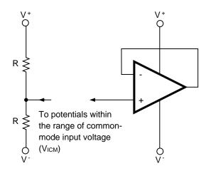
Remark: In this example, an intermediate potential between V<sup>+</sup> and V<sup>-</sup> is applied.
