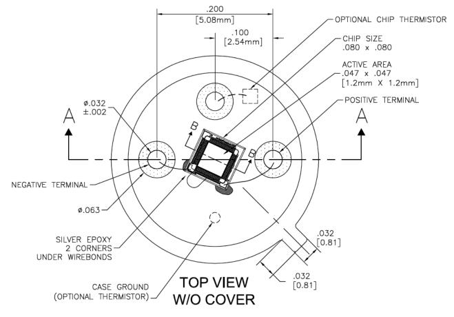
Figure 1. Package Outline Drawings – Top View
