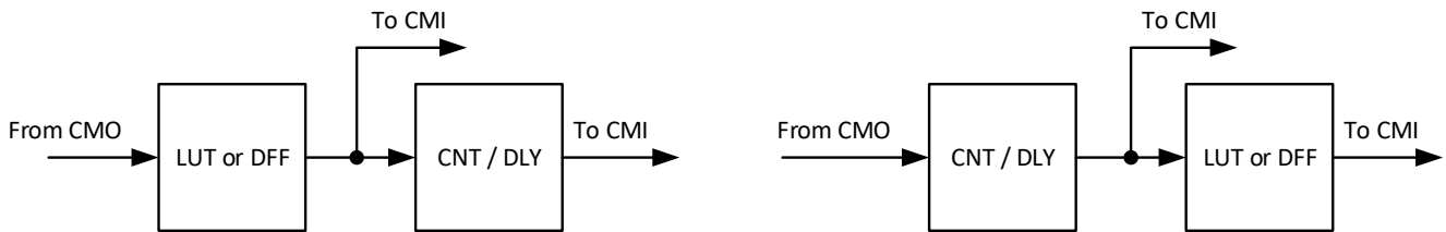
Figure 29. Possible Connections inside Multi-Function Macrocell
