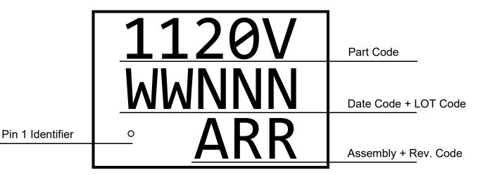
1120V - Part ID Field WW - Date Code Field<sup>1</sup> NNN - Lot Traceability Code Field<sup>1</sup> A - Assembly Site Code Field<sup>2</sup> RR - Part Revision Code Field<sup>2</sup>
