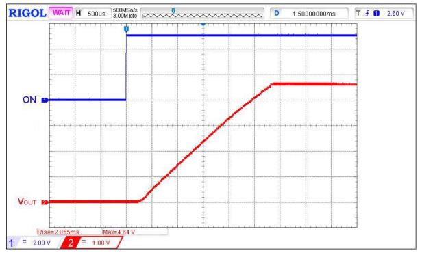
Figure 3. Typical Turn ON operation waveform for V<sub>IN</sub> = 4.5 V, C<sub>SLEW</sub> = 18 nF, C<sub>LOAD</sub> = 10  $\mu$ F, R<sub>LOAD</sub> = 100  $\Omega$
