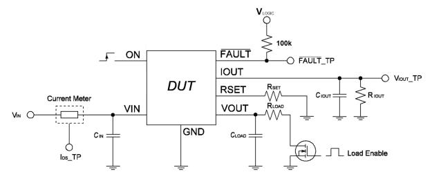
Figure 1. Test setup Application Diagram
