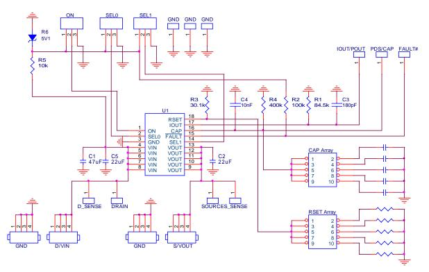
Figure 11. SLG59H1120V Evaluation Board Connection Circuit
