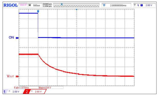
Figure 5. Typical Turn OFF operation waveform for V<sub>IN</sub> = 4.5 V, C<sub>SLEW</sub> = 10 nF, C<sub>LOAD</sub> = 10  $\mu$ F, R<sub>LOAD</sub> = 100  $\Omega$
