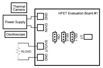
Figure 12. SLG59H1120V Evaluation Board Connection Circuit
