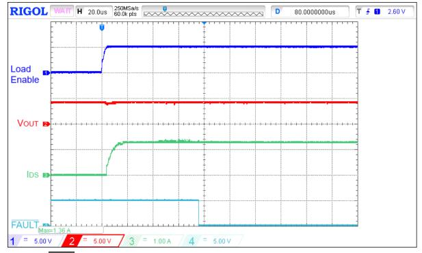
Figure 8. Typical FAULT assertion waveform for  $V_{IN}$  = 4.5 V,  $C_{LOAD}$  = 10 µF,  $I_{ACL}$  = 1 A,  $R_{SET}$  = 91 k $\Omega$ , switch on 3.3  $\Omega$  load
