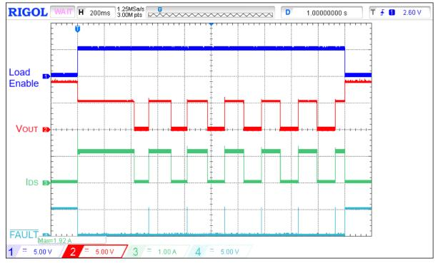
Figure 7. Typical ACL operation waveform for V<sub>IN</sub> = 9 V, C<sub>LOAD</sub> = 10  $\mu$ F, I<sub>ACL</sub> = 1 A, R<sub>SET</sub> = 91 k $\Omega$
