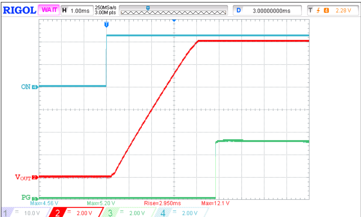
Figure 23. Turn ON and Power Good Operation Waveform for V_{IN} = 4.5 \text{ V}
