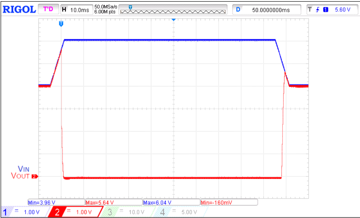
Figure 9. Typical Overvoltage Protection operation waveform for VIN step from 4 V to 6 V to 4 V, no R LOAD , no C LOAD
