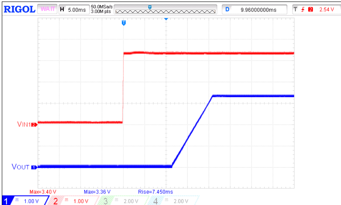
Figure 1. Typical Turn ON operation waveform for V_{IN1} = 3.3\text{ V} , C_{SS} = 220\text{ nF} , R_{LOAD} = 100\ \Omega , C_{LOAD} = 2\ \mu\text{F}
