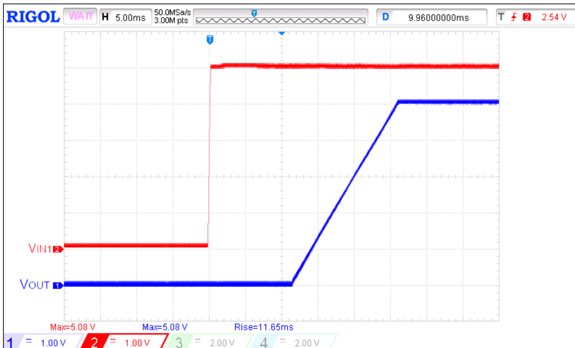
Figure 2. Typical Turn ON operation waveform for V_{IN1} = 5\text{ V} , C_{SS} = 220\text{ nF} , R_{LOAD} = 100\ \Omega , C_{LOAD} = 2\ \mu\text{F}
