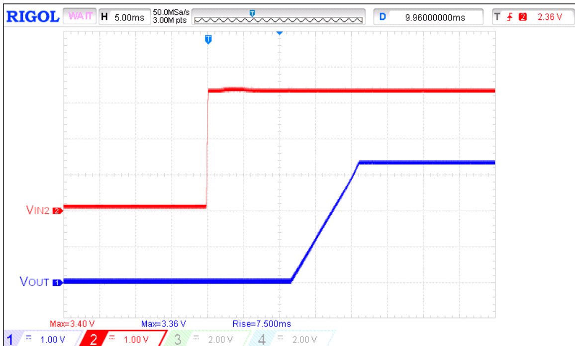
Figure 3. Typical Turn ON operation waveform for V_{IN2} = 3.3\text{ V} , C_{SS} = 220\text{ nF} , R_{LOAD} = 100\ \Omega , C_{LOAD} = 2\ \mu\text{F}
