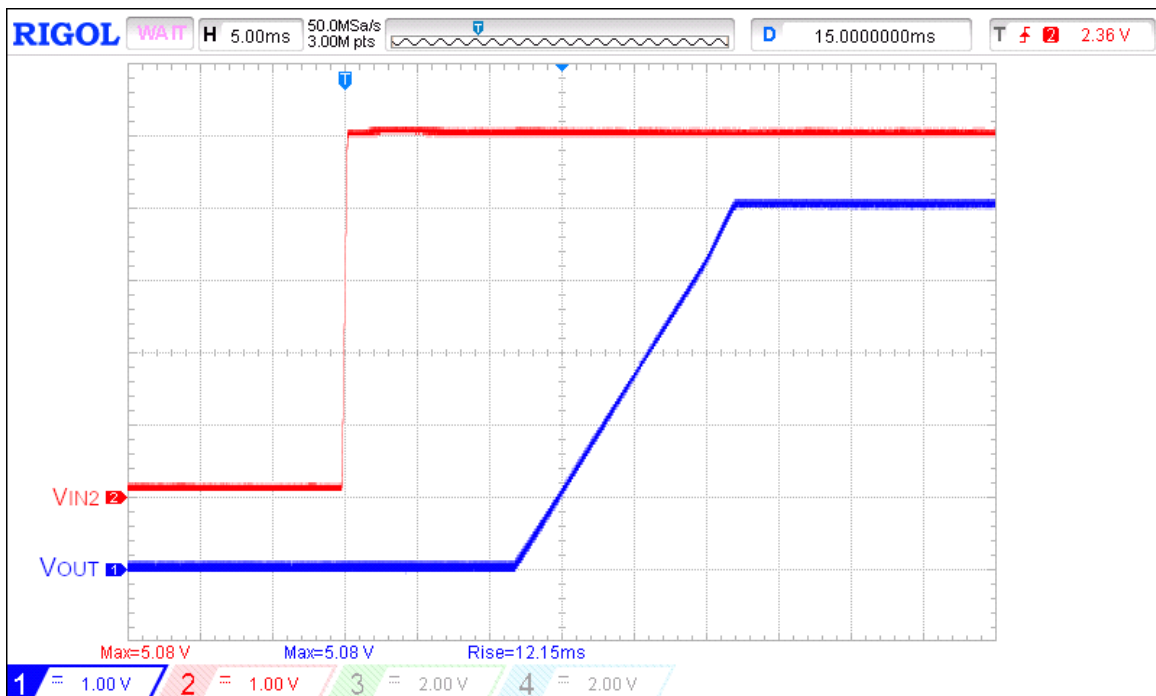
Figure 4. Typical Turn ON operation waveform for V_{IN2} = 5\text{ V} , C_{SS} = 220\text{ nF} , R_{LOAD} = 100\ \Omega , C_{LOAD} = 2\ \mu\text{F}
