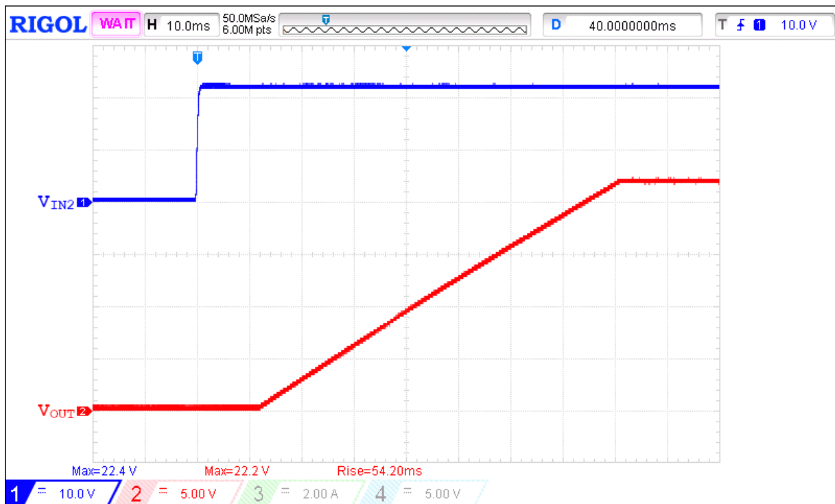
Figure 6. Typical Turn ON operation waveform for V_{IN2} = 22\text{ V} , C_{SS} = 220\text{ nF} , R_{LOAD} = 100\ \Omega , C_{LOAD} = 2\ \mu\text{F}
