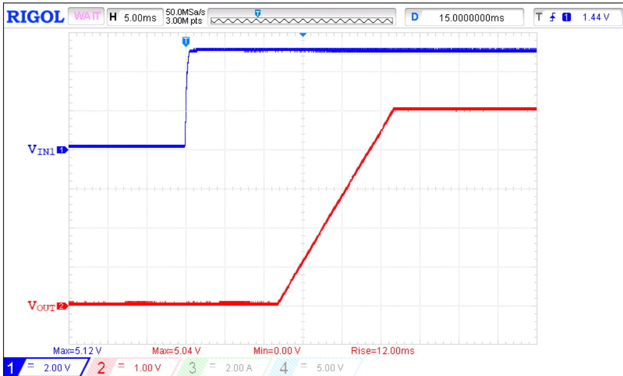
Figure 1. Typical Turn ON operation waveform for V_{IN1} = 5\text{ V} , C_{SS} = 220\text{ nF} , R_{LOAD} = 100\ \Omega , C_{LOAD} = 2\ \mu\text{F}
