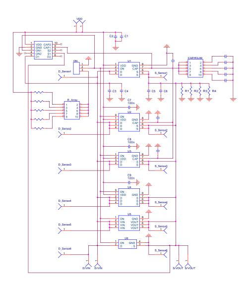
Figure 2. SLG59M1457V Evaluation Board Connection Circuit.
