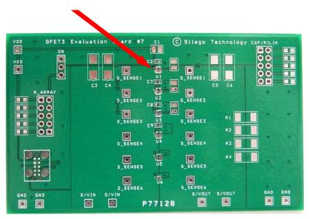
Figure 1. SLG59M1457V Evaluation Board.
