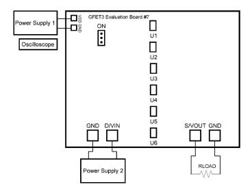
Figure 3. Typical connections for GreenFET Evaluation.
