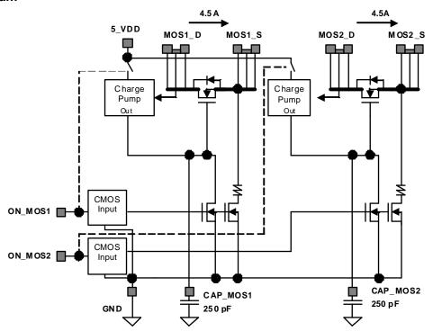
Do not probe CAP\_MOS1 (PIN 12) or CAP\_MOS2 (PIN 10) with low impedance probe.
