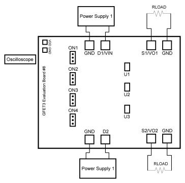
Figure 3. Typical connections for GreenFET Evaluation.
