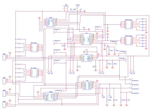
Figure 2. SLG59M1649V Evaluation Board Connection Circuit.
