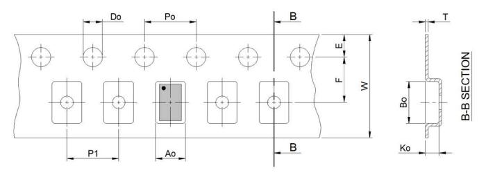
Note: Orientation in carrier: Pin1 is at upper left corner (Quadrant 1).
