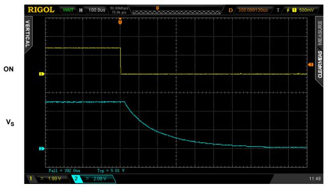
Figure 4. Typical Turn OFF operation waveform for V<sub>DD</sub> = V<sub>D</sub> = 5 V, C<sub>SLEW</sub> = 4 nF, C<sub>LOAD</sub> = 10 µF, R<sub>LOAD</sub> = 20  $\Omega$
