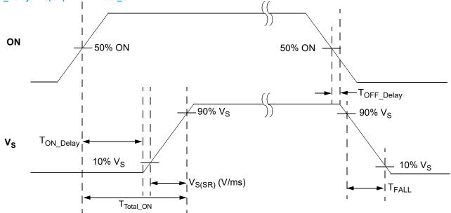
Note: Rise and Fall times of the ON signal are 100 ns
