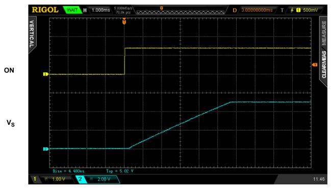
Figure 2. Typical Turn ON operation waveform for V<sub>DD</sub> = V<sub>D</sub> = 5 V, C<sub>SLEW</sub> = 12 nF, C<sub>LOAD</sub> = 10  $\mu$ F, R<sub>LOAD</sub> = 20  $\Omega$
