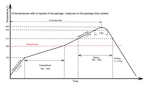
Note: This reflow profile is for classification/preconditioning and are not meant to specify board assembly profile. Actual board assembly profiles should be developed based on specific process needs and board designs and should not exceed parameters depicted on figure above.
