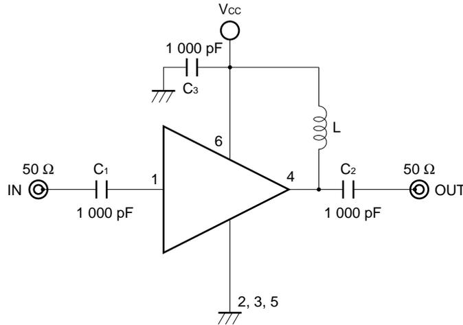
**COMPONENTS OF TEST CIRCUIT FOR MEASURING ELECTRICAL CHARACTERISTICS**
