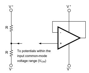
Note in this example, an intermediate voltage of V <sup>+</sup> and V <sup>-</sup> is applied.
