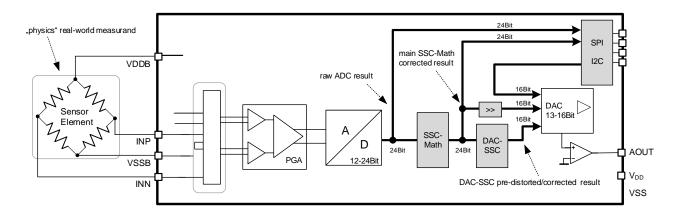
Figure 4. IC-Architecture View for Sensor-Signal-Transfer Perspective
