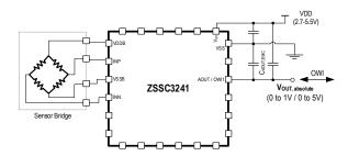
**Analog Sensor with Absolute Voltage Out**
