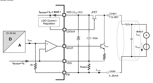
Figure 22. Current Loop Configuration
