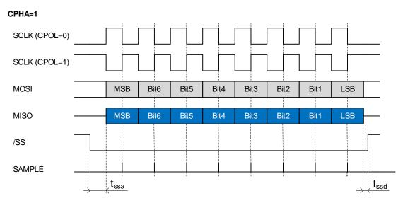
Figure 7. SPI Configuration CPHA=1
