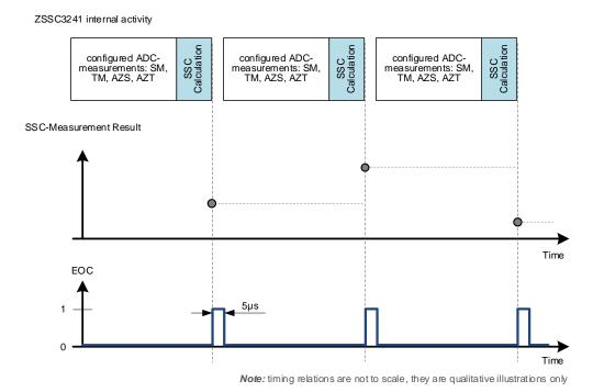
Figure 23. EOC-Behavior: Signalization of End-of-Conversion (INT\_setup = 00BIN)
