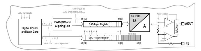
Figure 21. DAC and Analog Output Topology
