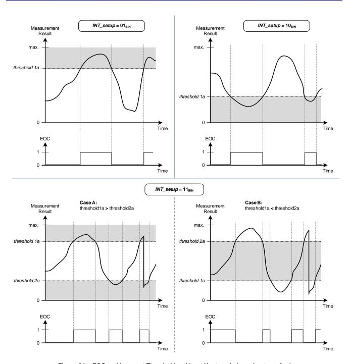
Figure 24. EOC and Interrupt Thresholds without Hysteresis (eoc\_hyst\_on=0<sub>BIN</sub>)
