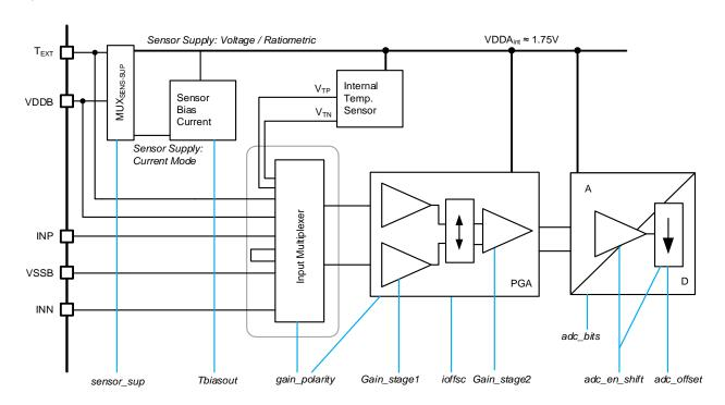
Figure 5. Analog Sensor Front-End Topology
