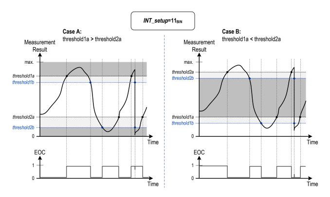
Always ensure that: threshold1b ≤ threshold1a and threshold2b ≤ threshold2a
