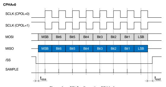
Figure 6. SPI Configuration CPHA=0
