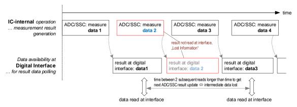
Figure 20. Measurement Result Output Update in Cyclic Operation (with "Slow" Interface Polling)
