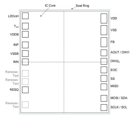
Figure 2. Pin (Pad) Assignments for Bare Die
