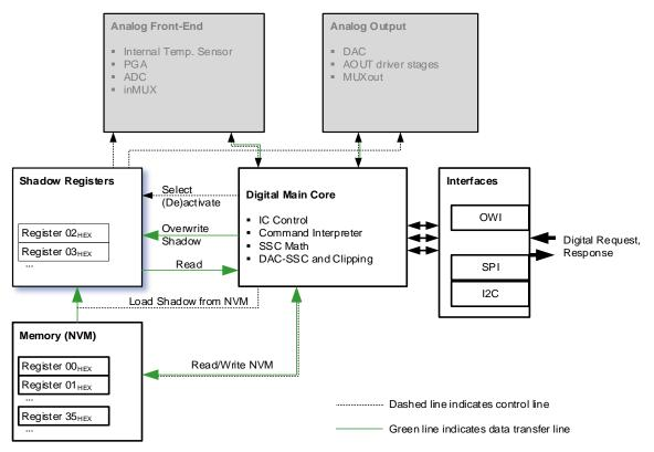
Figure 27. Digital IC Section Architecture
