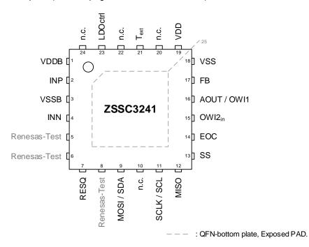
Figure 1. Pin Assignments for 4 × 4 mm<sup>2</sup> 24-QFN Package – Top View
