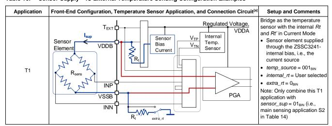
Table 16. Sensor Supply – IC External Temperature Sensing Configuration Examples
