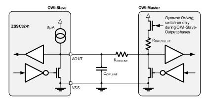
Figure 14. General Block Schematic of the OWI Interface
