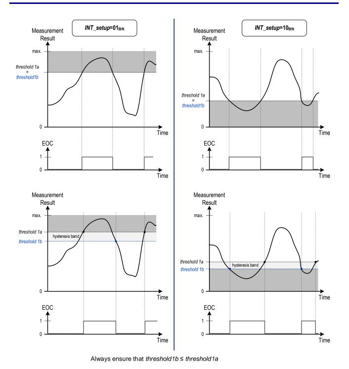
Figure 25. EOC and Single-Interrupt Thresholds with Hysteresis (eoc\_hyst\_on=1<sub>BIN</sub>)
