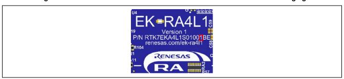
Figure 4. Identification of the Kit Version Number on the EK-RA4L1 Board.
