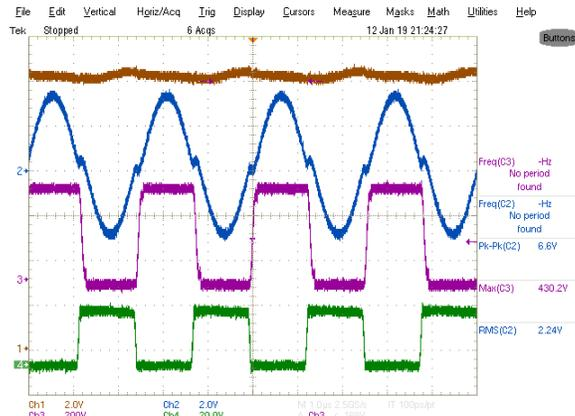
Fig. 10 Measured Efficiency Curve 385Vin-12Vo: CH1: Vo, CH2: IL, CH3: Vsw, CH4: VSR\_Mos
