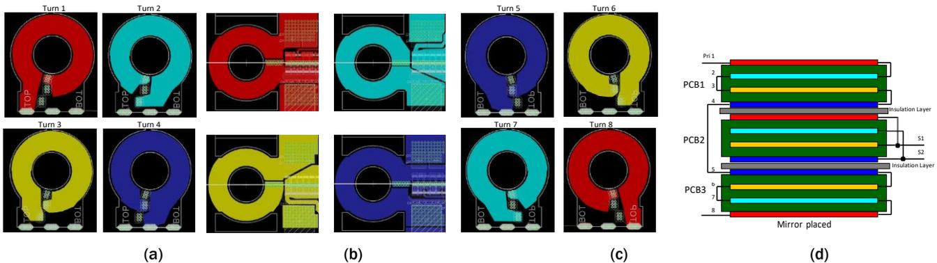
Fig. 5 PCB windings: (a) PCB1 layer1-4 as primary side 1<sup>st</sup> turn-4<sup>th</sup> turn; (b) PCB2 layer 1,3 as secondary side winding S1, 1 turn, layer 2, 4 as secondary side winding S2, 1 turn; (c) PCB3 layer1-4 as primary side 5<sup>th</sup> turn-8<sup>th</sup> turn. (d) PCB winding construction and connection
