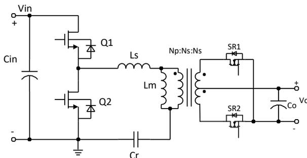
Figure 1. Schematic of half bridge LLC resonant converter.
