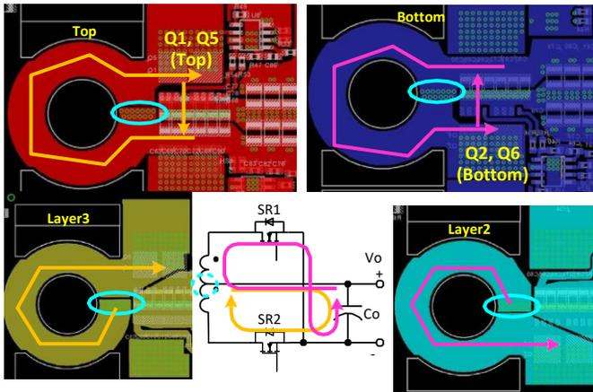
Fig. 6 Minimized secondary side circuit loop area
