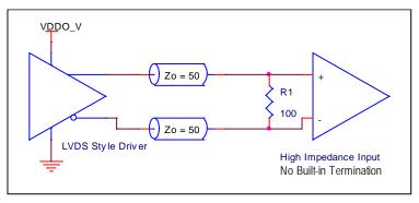
Figure 21. LVDS Style Driver Termination (DC Coupled)
