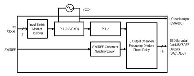
Figure 1. 8V19N882 Simplified Block Diagram
