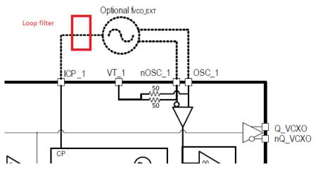
Figure 8. VCO PLL Block Diagram
