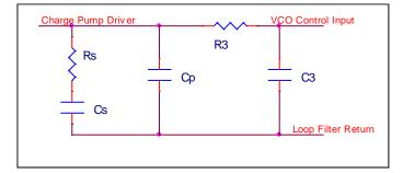
Figure 4. Typical 3<sup>rd</sup> Order Loop Filter
