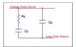
Figure 3. Typical 2<sup>nd</sup> Order Loop Filter
