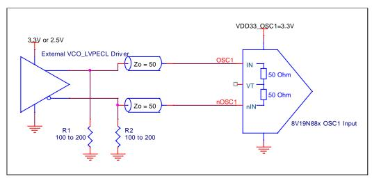
Figure 14. External VCO 3.3V LVPECL Driver to OSC\_1/nOSC\_1 Input, Alternative Interface
