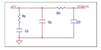
Figure 7. Typical 3rd Order Loop Filter
