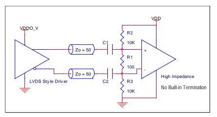
Figure 23. LVDS Style Alternative Driver Termination (AC Coupled)
