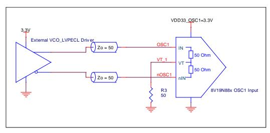
Figure 13. External VCO 3.3V LVPECL Driver to OSC\_1/nOSC\_1 Input Interface
