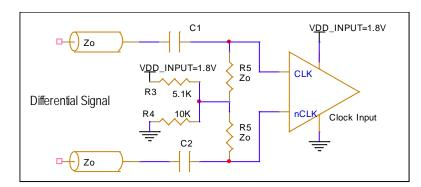
Figure 12. 8V19N882 Reference Clock Input CLK/nCLK AC Coupling Termination Example 2
