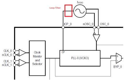
Figure 5. 8V19N88X VCXO Phase Lock Loop Block Diagram
