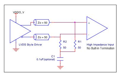
Figure 22. LVDS Style Alternative Driver Termination (DC Coupled)
