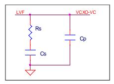
Figure 6. Typical 2<sup>nd</sup> Order Loop Filter
