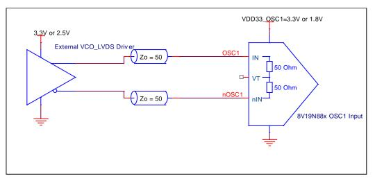
Figure 15. External VCO LVDS Driver to OSC\_1/nOSC\_1 Input Interface
