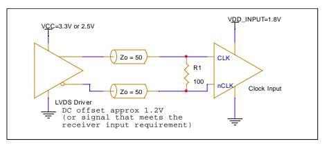
Figure 10. Input Termination Example – 8V19N882 Reference Clock Input CLK/nCLK Driven by an LVDS Driver
