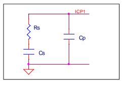
Figure 9. 2<sup>nd</sup> Order Loop Filter for the VCO
