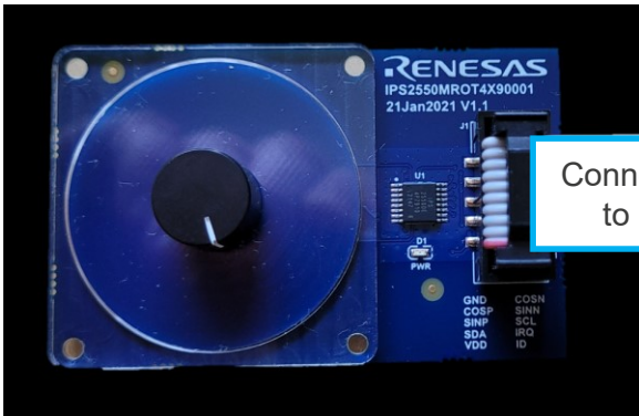
IPS2550 Sensor Module IPS2550MROT4X90001
