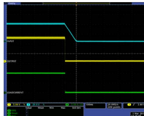
FIGURE 19. FULL LOAD SHUTDOWN, CH1: OUTPUT VOLTAGE, CH2: INPUT VOLTAGE, CH4: LOAD CURRENT
