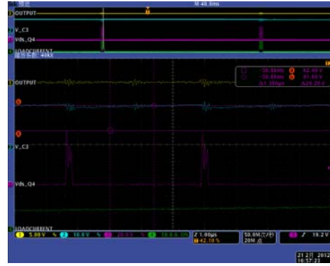
FIGURE 35. ZOOM IN, CH1: OUTPUT VOLTAGE, CH2: VOLTAGE ON C3, CH3: Vds OF Q4_SR, CH4: LOAD CURRENT
