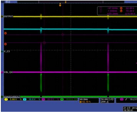
FIGURE 34. SHORT CIRCUIT, CH1: OUTPUT VOLTAGE, CH2: VOLTAGE ON C3, CH3: Vds OF Q4_SR, CH4: LOAD CURRENT
