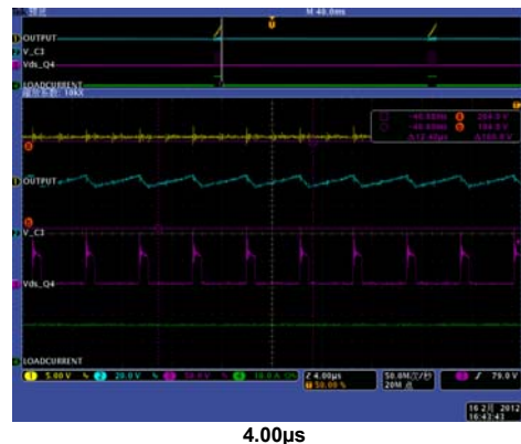
FIGURE 37. ZOOM IN, CH1: OUTPUT VOLTAGE, CH2: VOLTAGE ON C3, CH3: Vds OF Q4_SR, CH4: LOAD CURRENT
