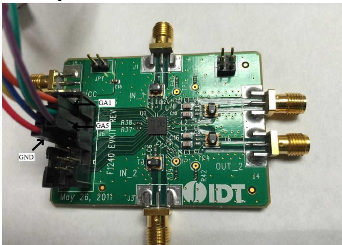
Figure 28. Parallel Mode Channel A Pin Connection for F1241EVB
