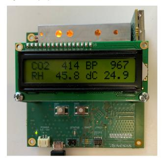
Two pushbuttons are used for viewing additional information and calibrating the board. **Sw1** cycles through displaying available modes and **Sw2** selects the currently displayed mode for further operations.
