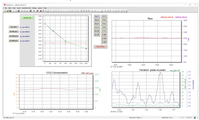
The EVK comes pre-calibrated, but it can be re-calibrated by the user if desired. CO<sub>2</sub> calibration can be performed in either of two ways:
