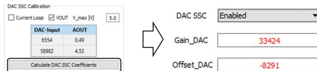
Figure 33. DAC SSC Calibration
