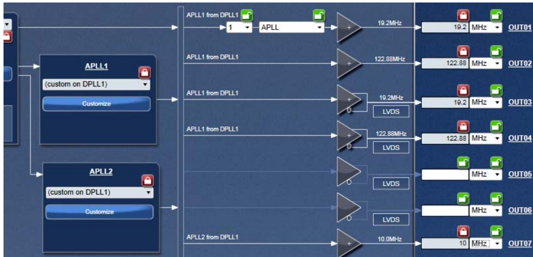
Figure 13. Output Frequencies Entered after APLL1/APLL2 Configured (example)
