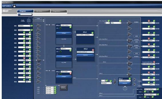
5. For Input configuration, most frequencies can be entered for IN01 ~ IN14 and they will be automatically configured to be available to both DPLLs.
