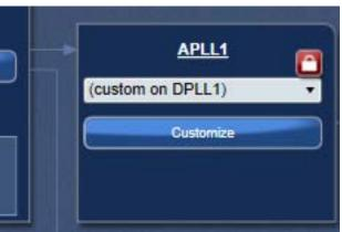
Click on the "Customize" button and ignore the initial Timing Commander error. Enter the values as shown in Figure 13 below to get a VCO of 614.4MHz.
