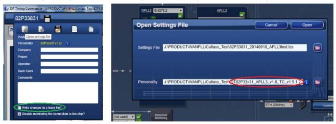
Once the same setting file and APLL-only personality file are selected, click on Open, a window for writing APLL3 will open, as shown below in Figure 21. Following the same procedure as shown in Figure 18 to connect and write to APLL3.
