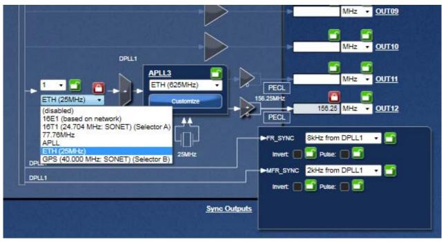
Finally, FRSYNC & MRFRSYNC can be configured, if needed. Change FRSYNC & MFRSYNC to 1PPS. By default, the duty cycle of sync outputs is 50/50. If a pulse is desired, click on the applicable check box. The pulse width is based on OUT01 clock period.
