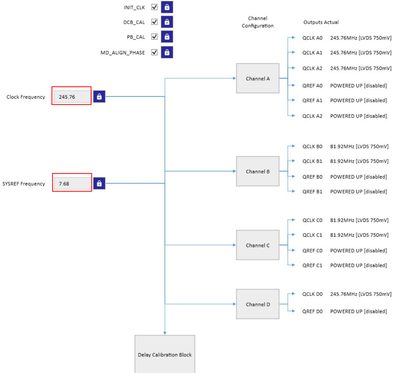
Figure 16. CLK/nCLK (Clock) and REF/nREF (Sysref) Input Frequency Setting
