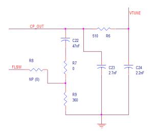
Figure 5. Loop Filter Schematic
