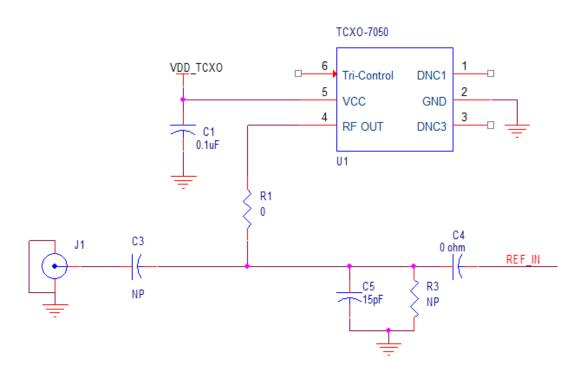
**Figure 4. Output Termination Schematic**
