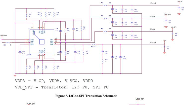
Figure 7. LDO Power Schematic
