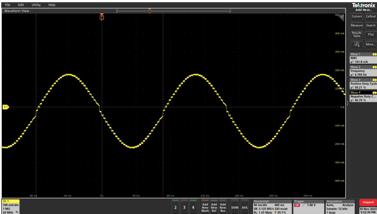
Figure 23: Current Waveform for Micro Step Mode
