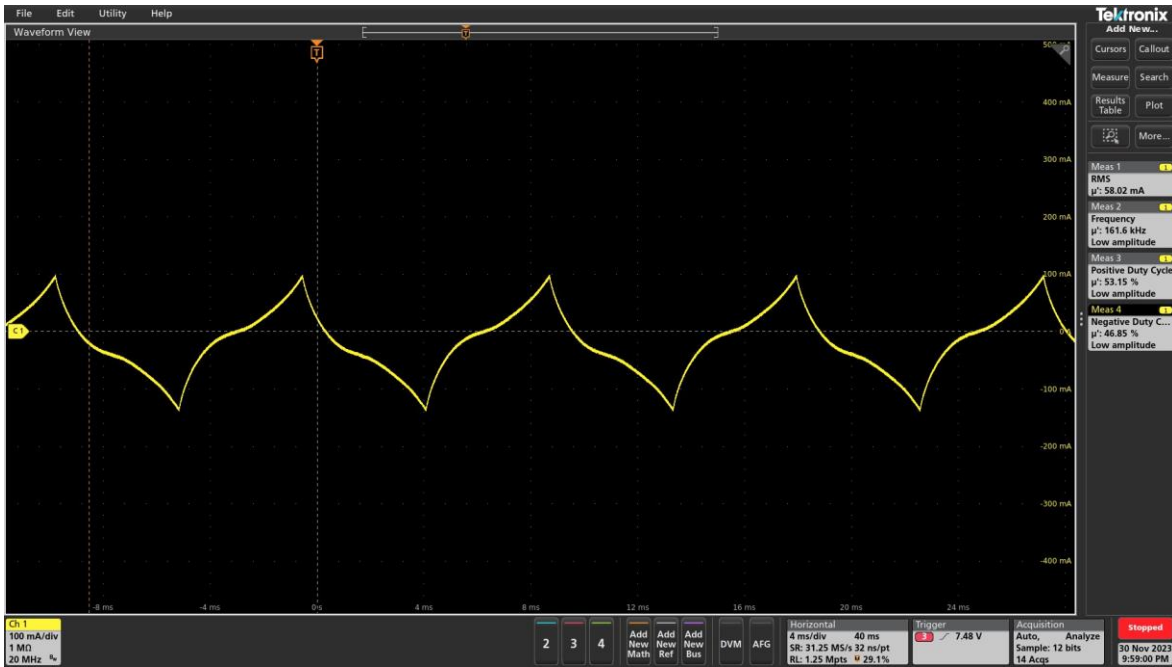
Figure 20: Current Waveform for Full Step Mode
