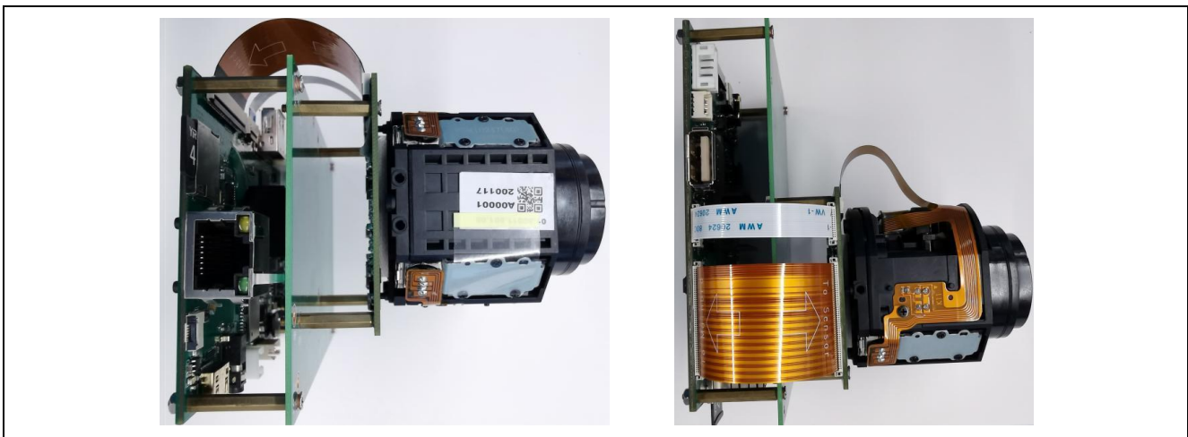
Figure 2.5 Mount ISP, CIS and Mounting Board
