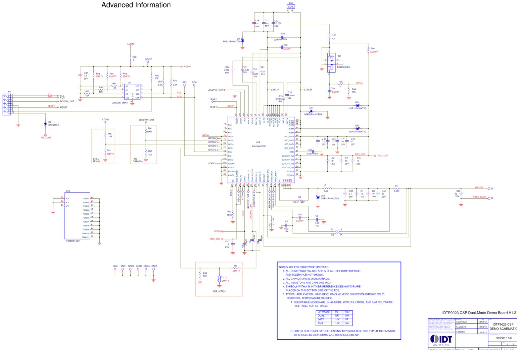
Figure 1. IDTP9023 V1.2 Eval Kit Board Schematic
