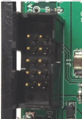
Figure 8. IDTP9023-EVAL JM60 Programmer input 10pin header.
