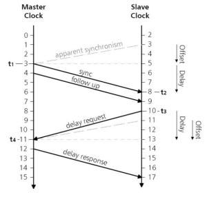
**Figure 1 PTP Basic Sync Operation**
