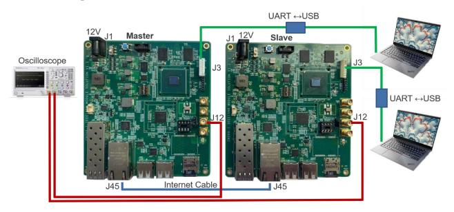
Figure 3 Quick Test Setup
