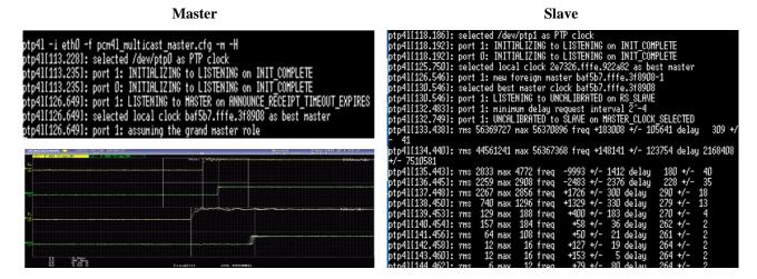
2. If want to stop slave PTP operation, for the first time after power on, please type "killall ptp4l" just like bellow, then using "Enter" Key of key board to confirm this line command.
