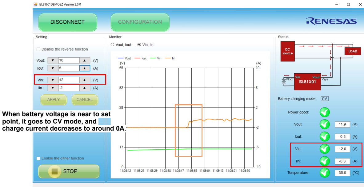
Figure 13. Fully Charging Information in GUI
