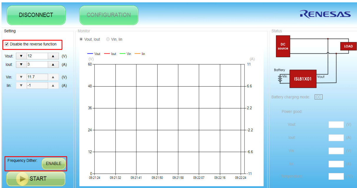
Figure 17. Disable Reverse Operation and Enable Dither Functions
