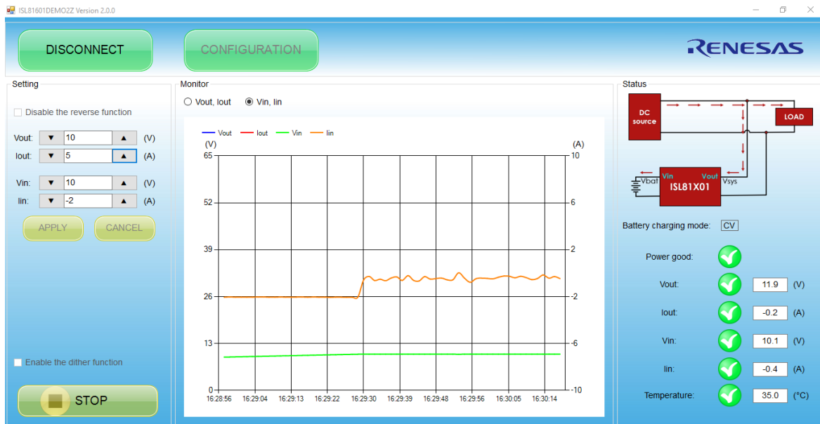
Figure 5. Fully Charged Information in GUI
